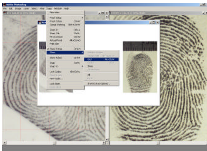
Figure 10. Enabling the Grid for alignment of callouts.
